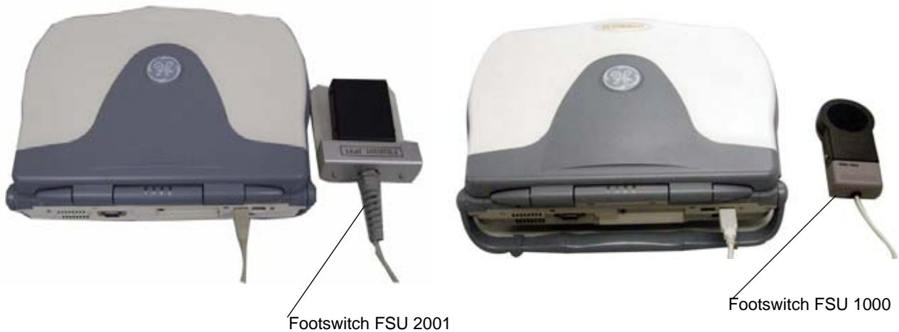
Figure 3-14 Connect Footswitch to the system
