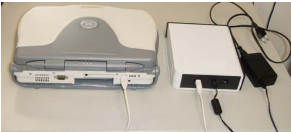
Figure 3-13 Connect CD-RW to the system
