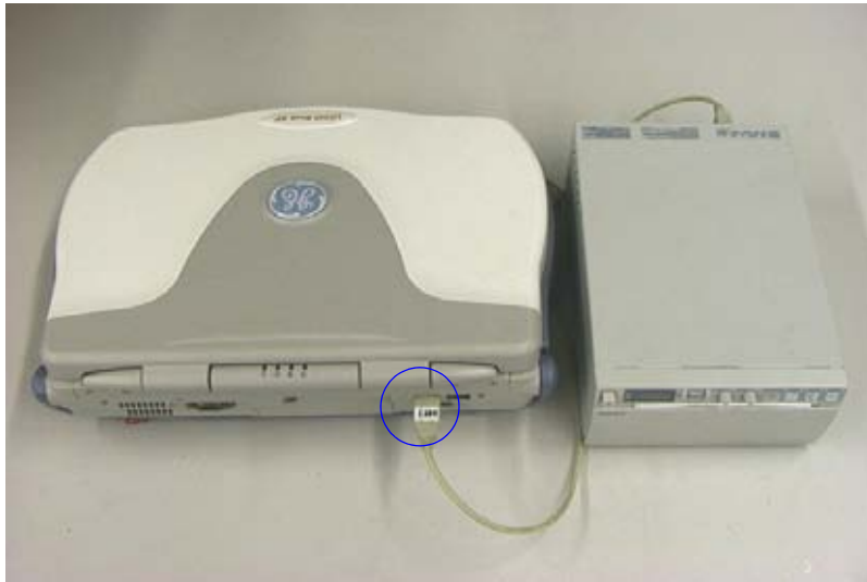
Figure 3-11 Connect B/W printer to the system
