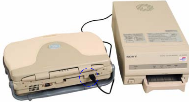
Figure 3-12 Connect digital color printer to the system
