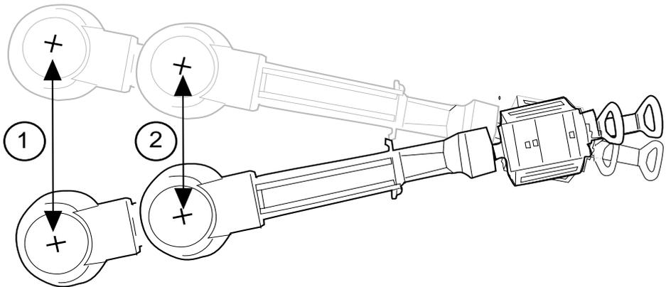
*Figure 4-11. Wig-Wag motion for a 23 cm (9-inch) system is shown.*
