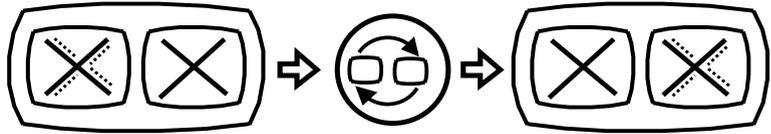
If the right monitor is blank, press the SWAP key to copy the image on the left monitor to the right monitor.
