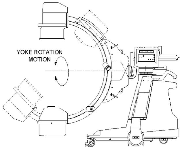
*Figure 4-5. Yoke rotation for 9-inch system*
