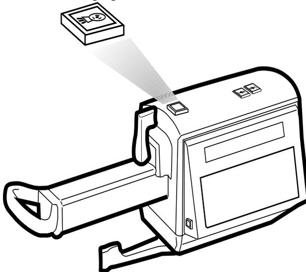
*Figure 3-4. The location of the X-ray on switch.*
