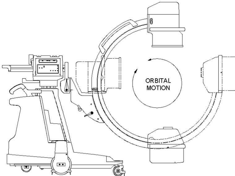
*Figure 4-3. C-arm Orbital Rotation for 9 inch*
