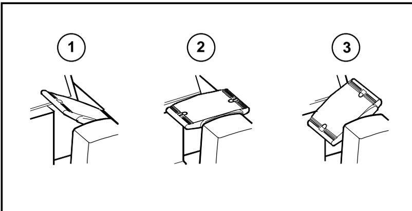
*Figure 4-13. C-arm brake pedal positions.*
