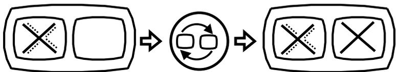
**After X-rays have been terminated** -the last frame of the exposure is retained on the left monitor (last image hold). Press the SWAP key to swap the images displayed on the left and right monitors.
