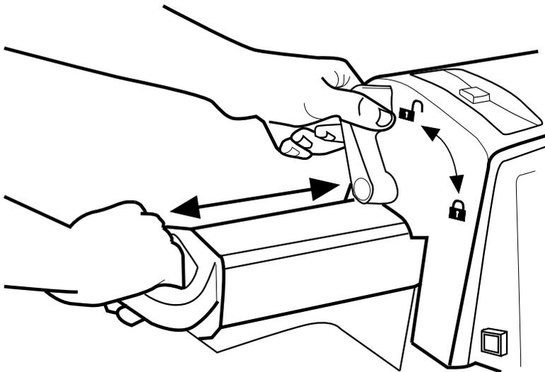
*Figure 4-10. The horizontal cross-arm brake.*
